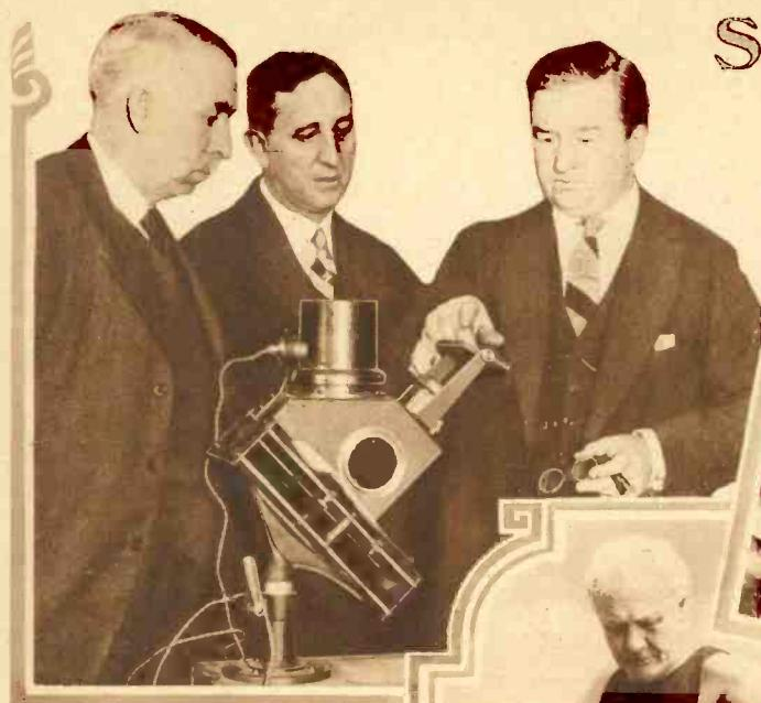
BEFORE science finishes, the life of the crook will be a hard one. Vide the Epidactyloscope, the latest bit of engineering brought to the aid of the police; the machine in spite of its long name is comparatively simple. It is nothing more or less than a device for enlarging finger-prints, so that the identification of criminals can be made swift and easy.
