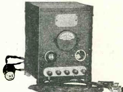
A distinctive advantage of this new vibrating rectifier is its ability to charge at varying rates as desired, up to 120 volts of "B" batteries in series. This eliminates the necessity of rewiring 24 volt sections in parallel in order to charge them. Two, 4, 6 or 8 volt "A" batteries may also be charged at a 5 to 7 ampere rate. The charger is furnished with meter, fuse plug, socket for lamp to vary "B" charging rate, 6 feet of lamp cord, and two charging wires, 4½ feet long.
