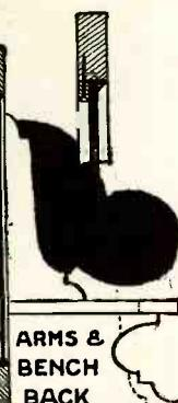
bench. We would suggest that the home mechanic construct his table to fit a standard size of porceliron top—40 inches x 32 inches, 40 inches x 24 inches, as examples. Make the table first and put it in place in the nook, then the benches having a length of 44 inches over all, and distances that are usable to any size and weight of person using this furniture. The furniture may be enameled either white or blue.
