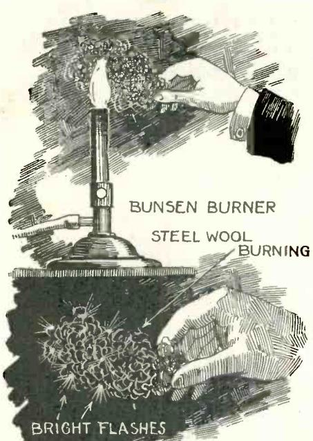
A piece of steel wool, if placed in the flame of a Bunsen burner for a second and removed, will emit bright flashes for about ten seconds. —Arthur A. Blumenfeld.
