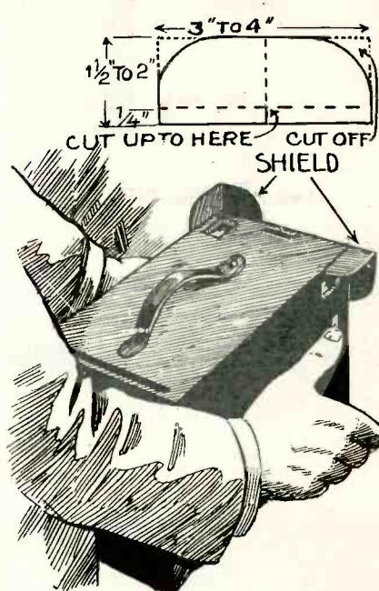
When using large hand cameras, it is often difficult to properly shield the finder with the hand so as to obtain a clear view. This difficulty can be overcome by cutting two shields from sheet tin in the shape shown above and attaching to the camera.
